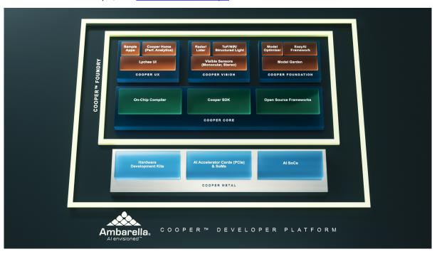
Cooper Metal is a hardware layer that includes power-efficient Al SoCs, Systems on Module (SoMs) and developer kits that come preloaded with Cooper Foundry.
