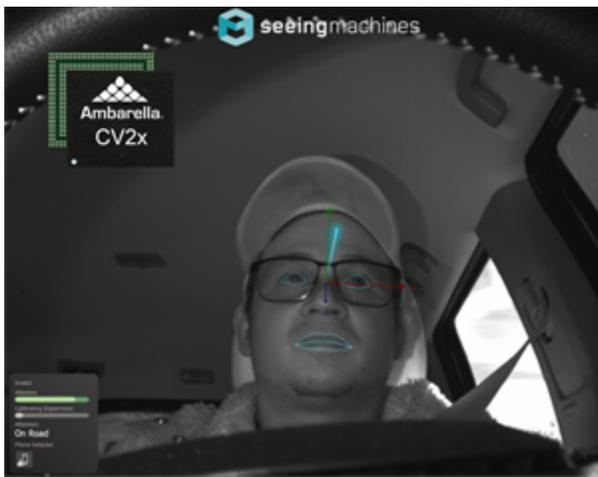
Ambarella's CV2x-based reference design platform performs the vision processing and fusion of Seeing Machines' driver monitoring software with forward-facing Advanced Driver Assistance System (ADAS) features to provide a complete, integrated driver monitoring system (DMS) and ADAS solution.
