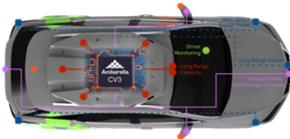
The Ambarella CV3 AI domain controller family enables centralized, single-chip processing for multi-sensor perception—including high-resolution vision, radar, ultrasonic and lidar—as well as deep fusion for multiple sensor modalities and AV path planning.
