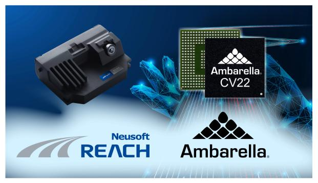
The third generation of Neusoft Reach's X-Cube 3.0 front view smart camera is based on Ambarella's CV22 AI vision system-on-chip (SoC), which runs the camera's L2 AI perception algorithm. The X-Cube 3.0 is currently being implemented in mass production, providing safe and efficient passenger car technologies and solutions for OEMs based on Ambarella's CV22 platform.
