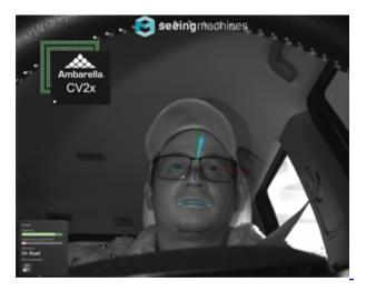
Ambarella's CV2x-based reference design platform performs the vision processing and fusion of Seeing Machines' driver monitoring software with forward-facing Advanced Driver Assistance System (ADAS) features to provide a complete, integrated driver monitoring system (DMS) and ADAS solution.
