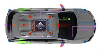
The Ambarella CV3 AI domain controller family enables centralized, single-chip processing for multi-sensor perception—including high-resolution vision, radar, ultrasonic and lidar—as well as deep fusion for multiple sensor modalities and AV path planning.
